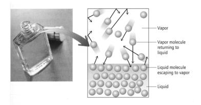
Boiling Point: Temperature at which the vapor pressure of the liquid equals the atmospheric pressure
