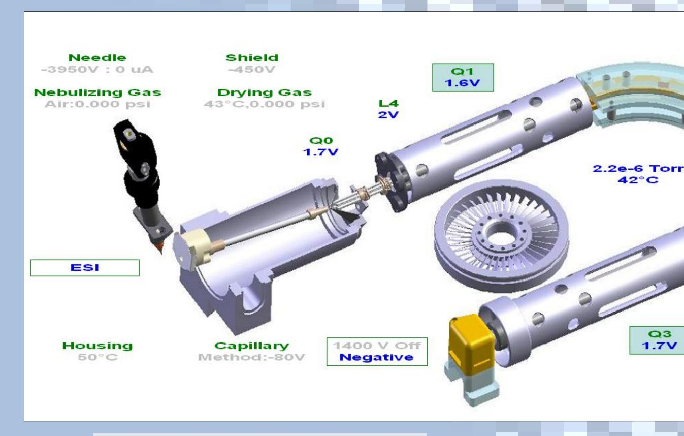
Figure 3. Diagram of the ESI-MS/MS utilized in the LC-MS
